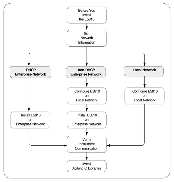
Installing the E5810 Installation Flowchart
