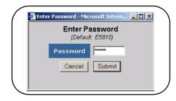
If the default password (E5810) is being used, the password is displayed as asterisks (\*\*\*\*\*). If not, type in the current password. Then, click the **Submit** button to display the **Configuring Your E5810 LAN/GPIB Gateway** page.
