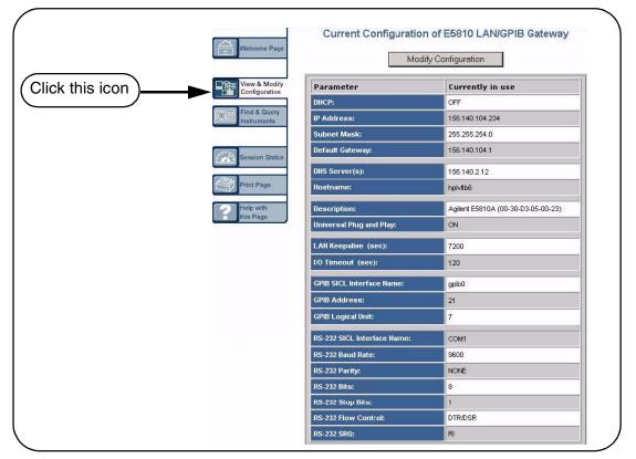
3 Display the Modify Configuration Page. From the Current Configuration of E5810 LAN/GPIB Gateway page, click the Modify Configuration button to display the Password dialog box.
