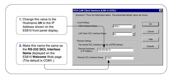
4 Do Not Delete the LAN Client Interface. When the VISA LAN Client is configured, the LAN Client is also automatically configured in the background. Thus, when VISA LAN Client configuration completes, two configured interfaces are displayed on the IO Config main screen. See the following figure for a typical display. Do NOT remove the LAN Client or VISA LAN Client interface, as the application will not run if either interface is removed
