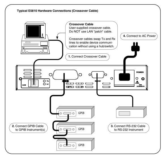
Apply Power to the E5810 After connecting the E5810 to a Local network, plug the E5810 AC power cord into an AC outlet and observe the power-on sequence. When the power-on sequence is complete, the default IP address of the E5810 is displayed on the second line of the front panel display. A typical display follows. See *Chapter 1 - E5810 Description* for power-on sequences.
